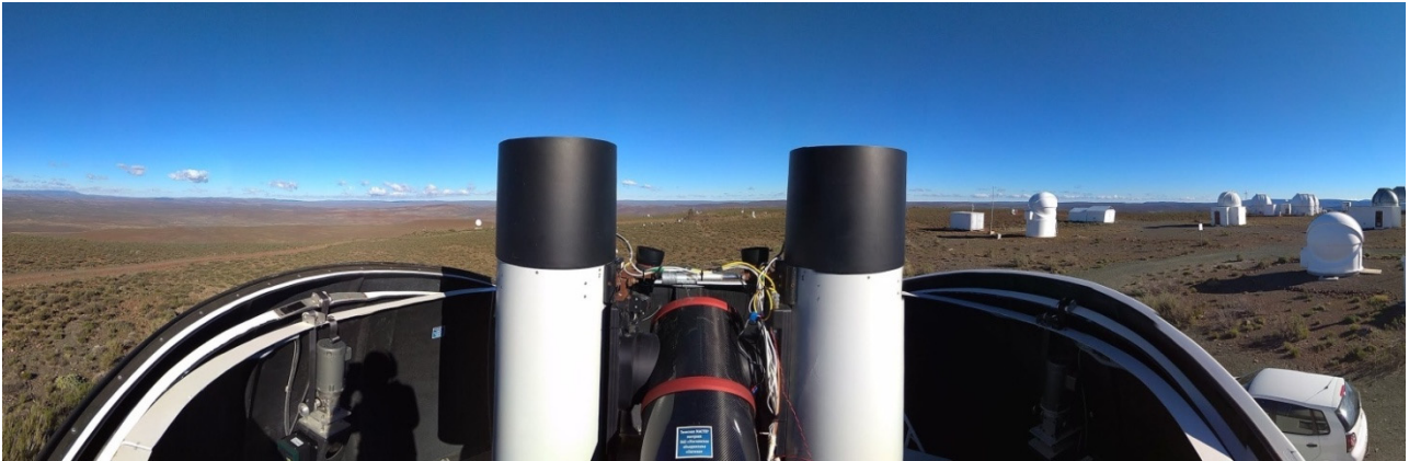
Figure 2. MASTER-SAAO telescope-robot at the South African Astronomical Observatory (SAAO) near Sutherland. Typical design: two 400 mm tubes with a 2 \times 4 square degrees field of view and two very wide-field view cameras (VWFC with FOV = 2 \times 384 square degrees) at fast mount. The Figure was taken from http://observ.pereplet.ru/ (accessed on 1 March 2021).
