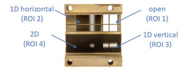
**Figure 3.** The optical-collimator element of the payload consisting of four segments of distinct response, see text. Size of the entire element  $26 \text{ mm} \times 24 \text{ mm} \times 11.4 \text{ mm}$  (height) (see Figure 1).
