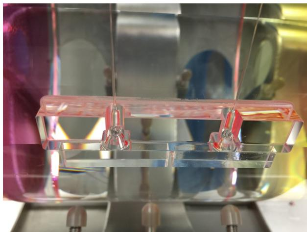
**Figure 6.** Mirror suspension of fused silica fibers. Two fibers are welded to rectangular silica pieces anchored to another silica rectangular block which in turn is attached to flats worked out in the mirror lateral surface. All the silica surfaces are attached by hydroxide-catalysis bonding. Credit: The Virgo Collaboration.
