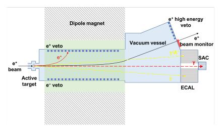
**Figure 4.** Schematic, top view of the PADME detector. The main components are indicated together with the tracks corresponding to a Bremsstrahlung event (red) and a  $\gamma\gamma$  event (yellow) (see text for more details).
