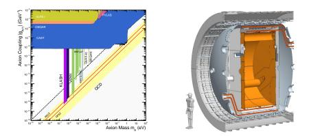
**Figure 3. Left**: the KLASH discovery potential compared to existing experimental limits. **Right**: a section view of the KLOE magnet surrounding the cryostat with its radiation shield and the copper cavity.
