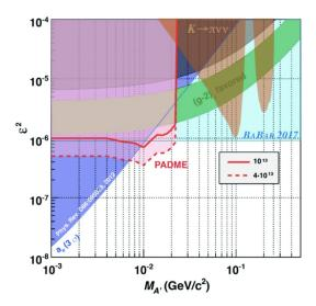
**Figure 5.** PADME exclusion region of the parameter space ( $\varepsilon^2$ ,  $M_{A'}$ ) for different values of the integrated luminosity.
