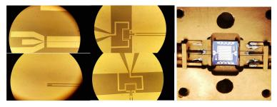
**Figure 2. Left**: optical image of the RF-chip with JJ and DC-SQUID fabricated at CNR-IFN for the SIMP project. **Right**: TWJPA from INRiM inside the LNF sample holder before bonding.
