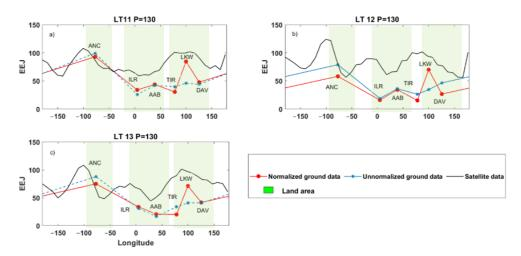
**Figure 4.** The longitudinal variation of the EEJ current derived from the ground (nT) and satellite (mA/m) data during high solar activity level (P = 130) at (a) 11 LT (b) 12 LT, and (c) 13 LT.
