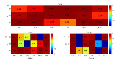
**Figure 5.** The computed correlation coefficient (*r*) between satellite and ground data at 11 to 13 LT during (**a**) low (P = 70), (**b**) moderate (P = 98) and (**c**) high (P = 130) solar activity level.
