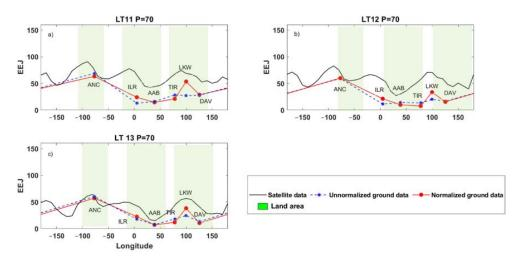
**Figure 2.** The longitudinal variation of the EEJ current derived from ground (nT) and satellite (mA/m) data during low solar activity level (P = 70) at (a) 11 LT (b) 12 LT and (c) 13 LT.
