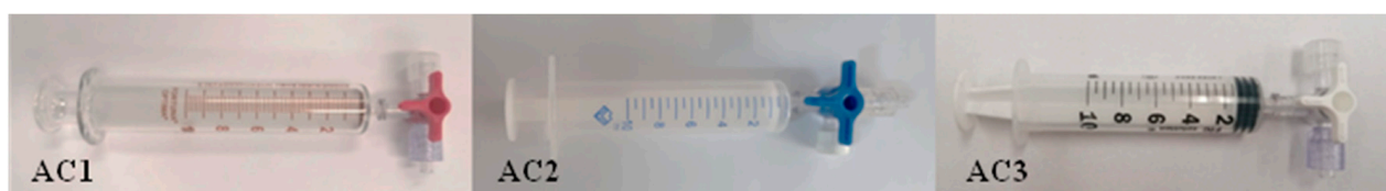
Figure 1. Syringe-based Air Containers (AC) used in the study: full glass (AC1, left), plastic with plastic plunger (AC2, middle) and plastic with rubbered plunger (AC3, right).
