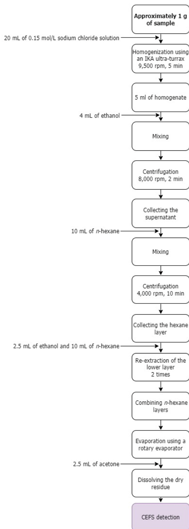
Figure S4. Workflow of the analytical method adapted from Román-Pizarro et al., 2017.
