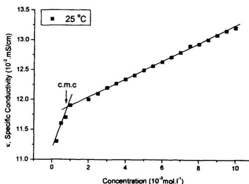
**Fig. 1.** Electrical conductivity vs. HCC XIX concentration
