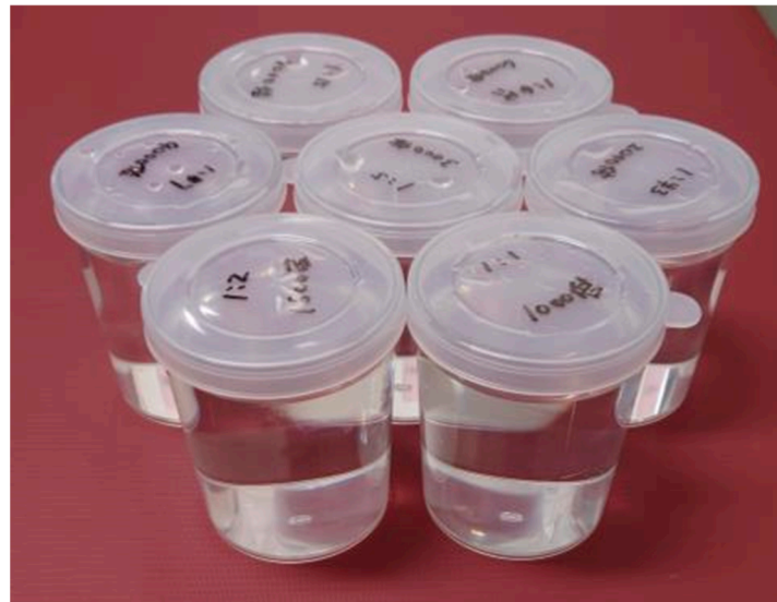
Figure 1. A photograph of the phantoms. Seven phantoms were made by mixing Gd-DOTA and water and sealing them in polypropylene cylinder-shaped containers (diameter, 6 cm; height, 8 cm).
