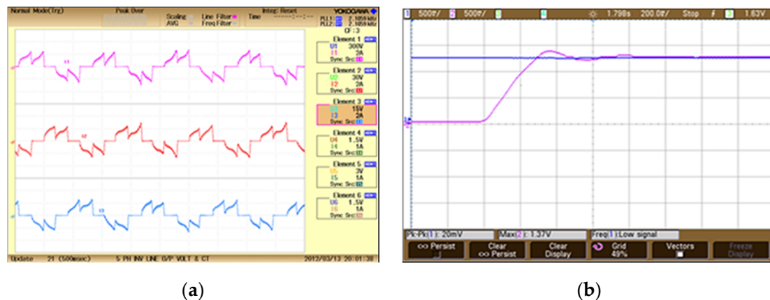
Figure 16. The brushless motor (a) current and (b) speed waveform.
