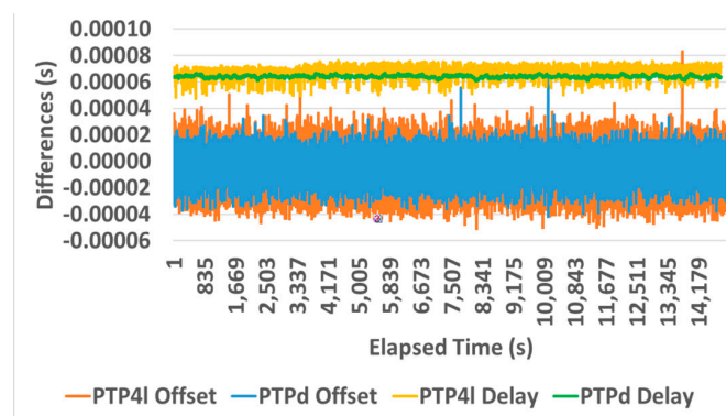
Figure 2. Offset and delay range of two PTP daemons running on the same machine.
