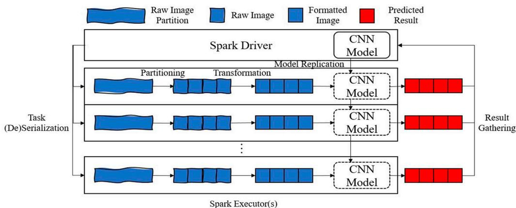
Figure 1. Processing procedure of Spark CNN based on model replication-based data parallelism.
