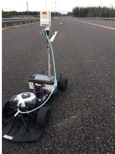
Figure 10. UWB mobile node attached to the RC car.
