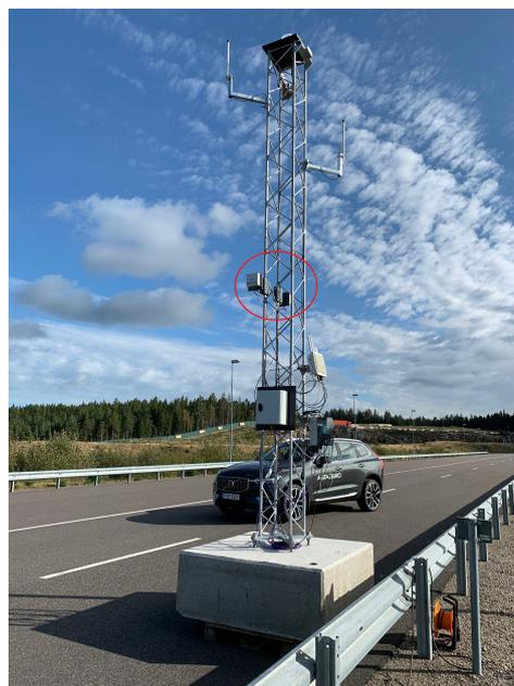
Figure 8. A couple of UWB anchor nodes installed at one gantry pole in the Astazero proving ground.
