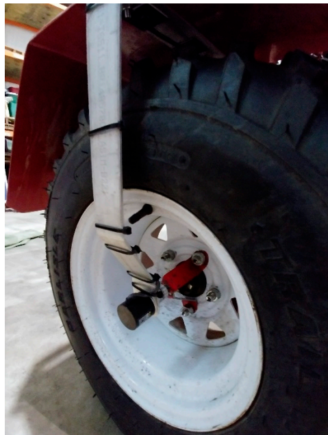
Figure 5. Encoder installed on the front tire of the rover to provide input pulses, which indicate how far the rover has moved.
