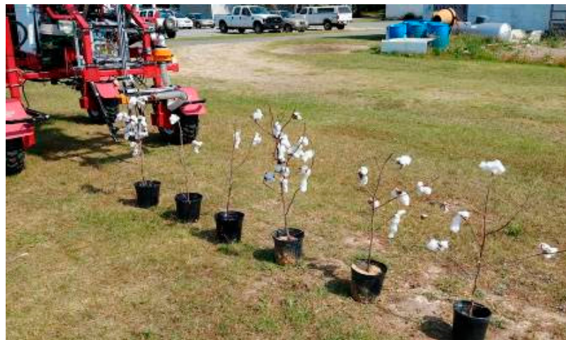
Figure 17. The experiment was set up at University of Georgia (UGA) grounds, to test the robot on picking the bolls in a simulated environment consisting of six potted cotton plants.
