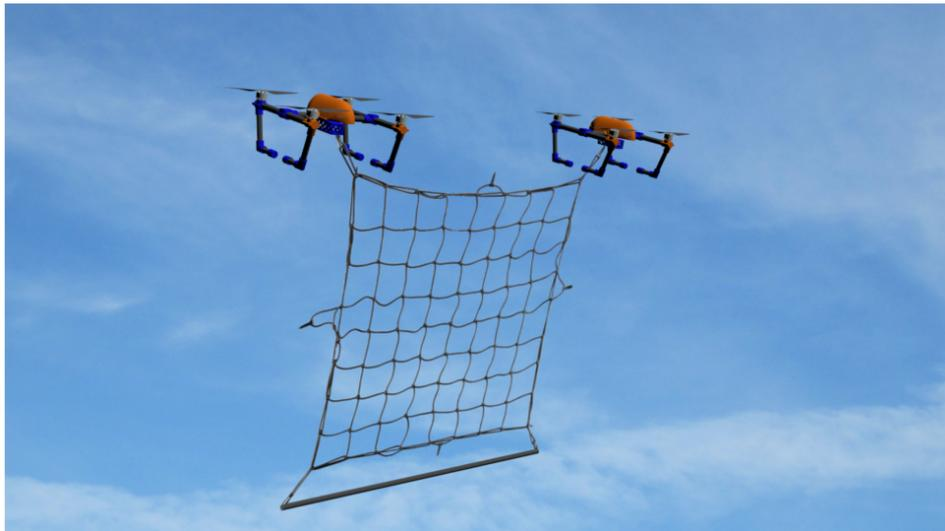
**Figure 1.** Model of the UAV system carrying a net.
