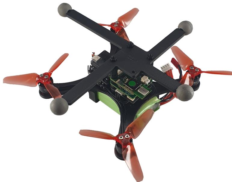
**Figure 8.** Micro-UAV with optical markers used for the evaluation.
