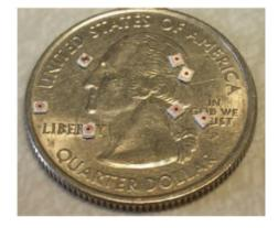
Figure 2. Manufactured measuring cups for the filling of magnetic particles in the MRS cavities.
