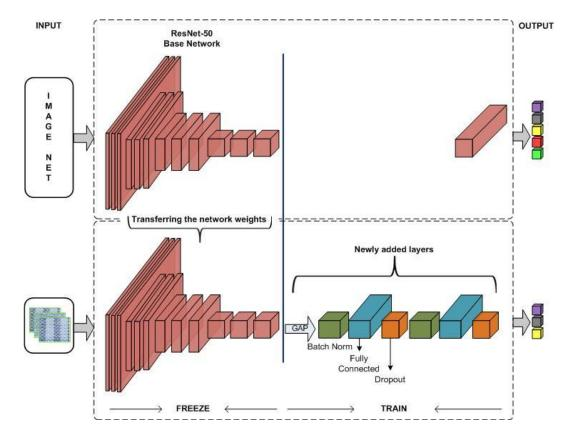
Figure 6. Overall framework of the proposed model.
