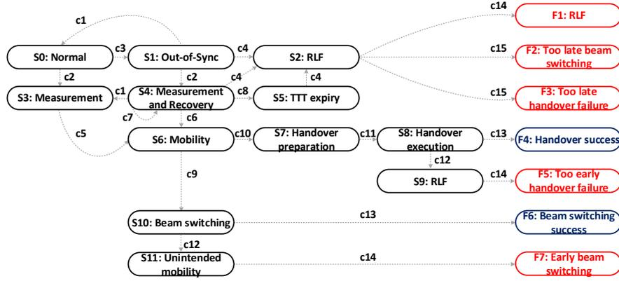
Figure 3. User finite state machine for proposed scheme.
