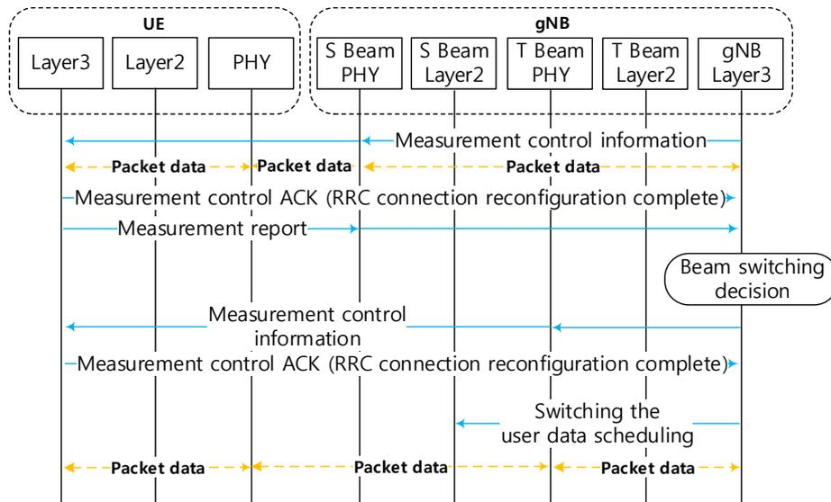
Figure 2. Beam switching process in the proposed scheme.
