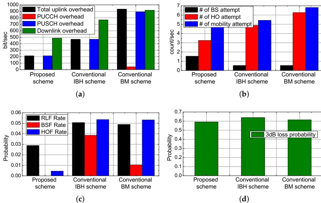
**Figure 5.** Results under the UDN scenario. (a) overhead performance, (b) mobility attempts, (c) mobility failure rates, (d) 3-dB loss probability.
