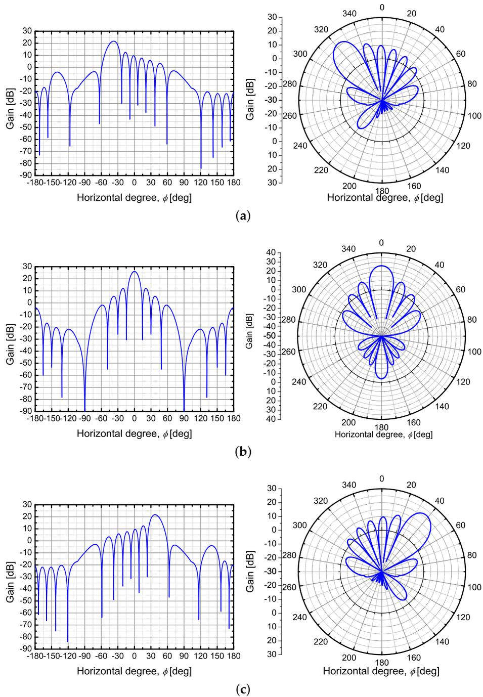
**Figure 1.** Example of the beam pattern in relation to  $L = 3$  case. (a) beam pattern configuration in Cartesian (left plot) and polar (right plot) coordinate systems with  $G_t(0)$ , (b) beam pattern configuration in Cartesian (left plot) and polar (right plot) coordinate systems with  $G_t(1)$ , (c) beam pattern configuration in Cartesian (left plot) and polar (right plot) coordinate systems with  $G_t(2)$ .
