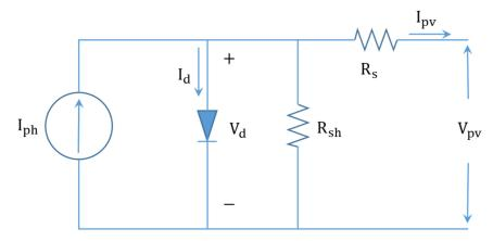
Figure 1. Equivalent of solar cell.
