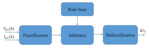
Figure 12. Variable step using Fuzzy control II.
