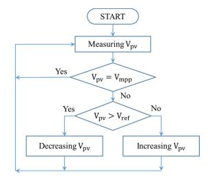
Figure 2. Flowchart of CV method.
