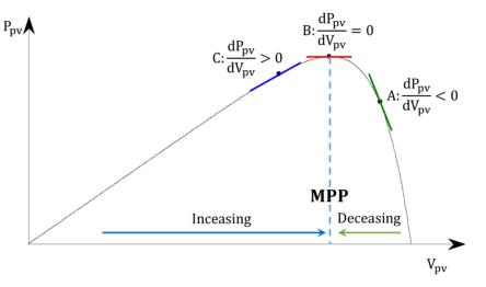
Figure 13. P-V curve and slope conditions.
