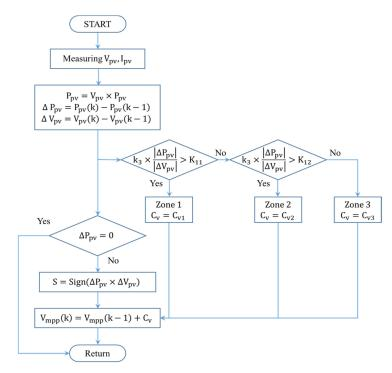
Figure 9. Flowchart of the modified P&O method.
