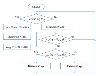
Figure 4. Flowchart of OCV Method.
