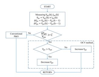
Figure 17. Flowchart of the P&O and OCV combination method.
