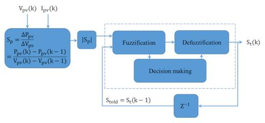
Figure 11. Variable step using Fuzzy control I.
