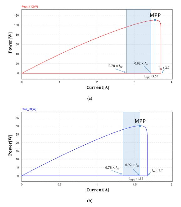
Figure 5. P-I curve of PV module. (a) PV module: 110 Wp; (b) PV module: 30 Wp.
