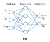
**Figure 16.** Neural network configuration by inputs (**a**) Electrical input; (**b**) Non-electrical input; (**c**) Combined electrical and non-electrical input.
