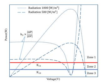
Figure 8. Changing value (C<sub>v</sub>) and Zones 1~3 in the P-V curve.
