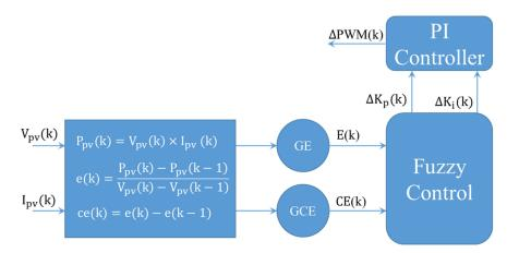
Figure 18. PI controller and Fuzzy control combination method.
