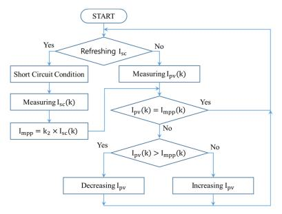
Figure 6. Flowchart of SCC method.
