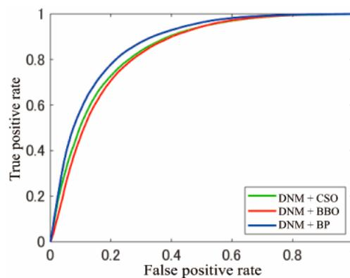
**Figure 9.** Receiver operating characteristic (ROC) of each method in F1.
