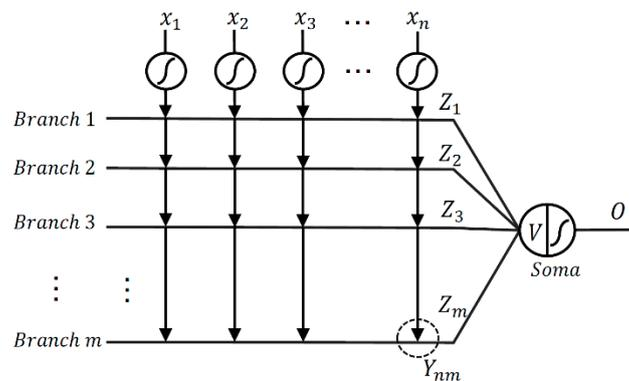
**Figure 1.** Structure of the dendritic neuron model (DNM).
