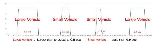
Figure 9. Threshold to classify vehicle types.
