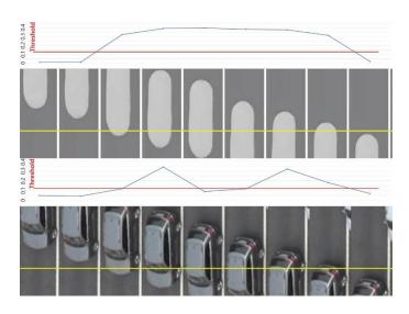
Figure 8. Signal profile comparison between a real vehicle (bottom) and a synthesized vehicle shape (top).
