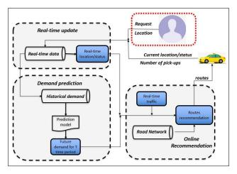
**Figure 1.** Recommendation framework for regular (without red curved rectangle) and ride-hailing (with red curved rectangle) taxi services.
