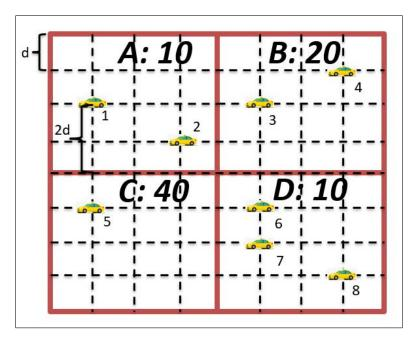
**Figure 5.** An illustrative example of an  $8 \times 8 d^2$  area composed of four regions A, B, C, and D with different demands 10, 20, 40, and 10, respectively. Eight vacant taxis are circulating around the region. The black dashed lines represent roads.
