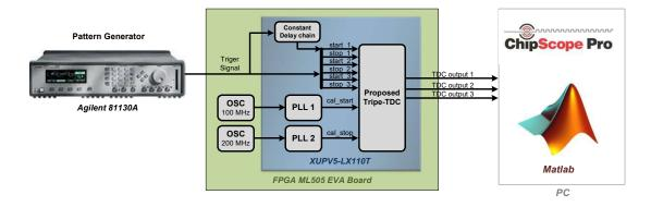
Figure 6. Measurement environment of this work.
