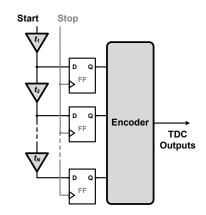
Figure 1. Architecture of the traditional TDL-TDC.
