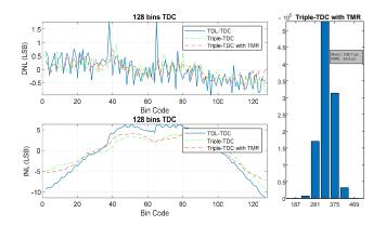
Figure 9. Measured INL, DNL, and RMS values for the proposed triple-TDC with TMR.
