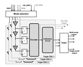
Figure 3. Architecture of the proposed triple-TDC.
