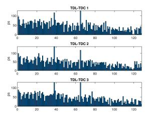
Figure 2. Time distribution for three TDL-TDCs.
