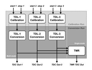
Figure 5. Operation flow of the proposed triple-TDC.
