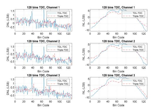
Figure 7. Measured DNL and INL values for the triple-TDC and TDL-TDC.
