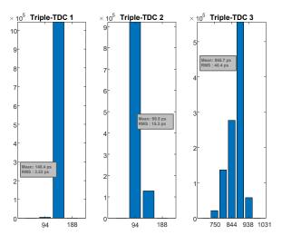
Figure 8. Measured RMS values for the proposed triple-TDC.
