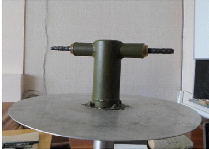
**Figure 1.** View of the dipole antenna operating at 600 MHz with its radiation elements made from carbon fiber.
