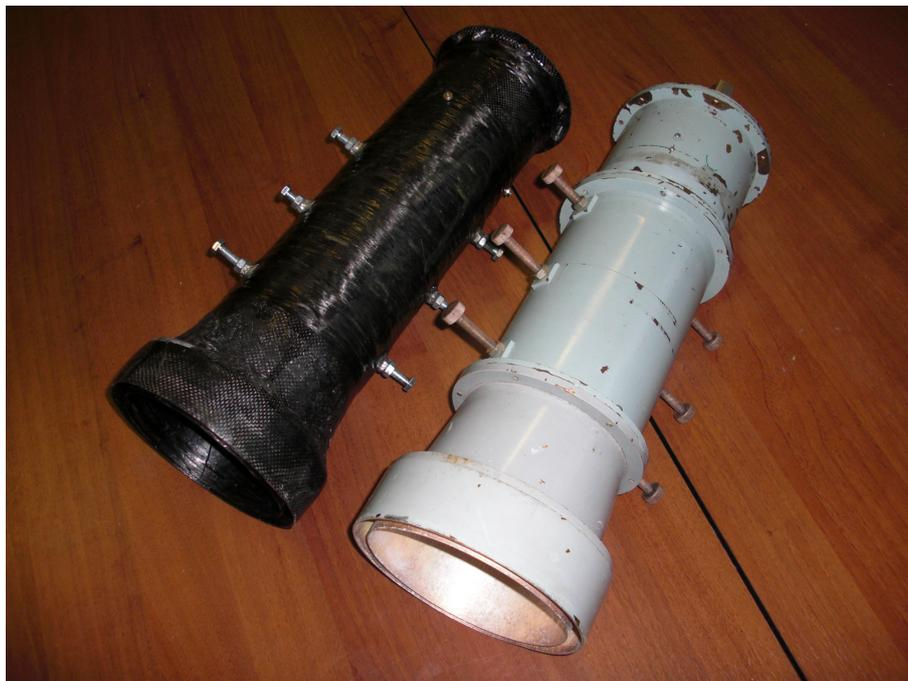
**Figure 8.** View of *L*-range horn antennas with polarization units made from fiber (left) and metal (right).
