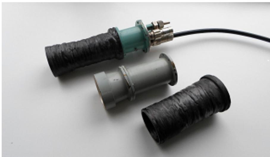
Figure 7. View of *C*-range horn antennas made from fabric (right), metal (center) and fiber (equipped with elements for antenna feeding, left).
