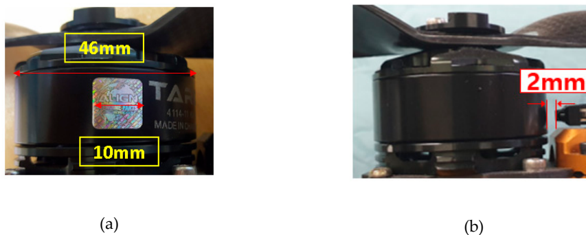
Figure 4. Measuring the rotational speed of the motor using the infrared sensor. (a) Diameter of motor and length of reflector; (b) the distance between the reflector and the infrared sensor.
