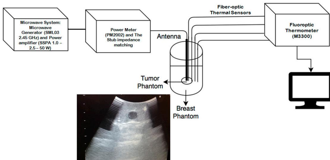
**Figure 2.** Phantom Experimental Setup. The radiation system supplied the microwave power to generate thermal ablation, while the non-interfering thermometry system measured the temperature increases inside the phantom every second during the experimentation.
