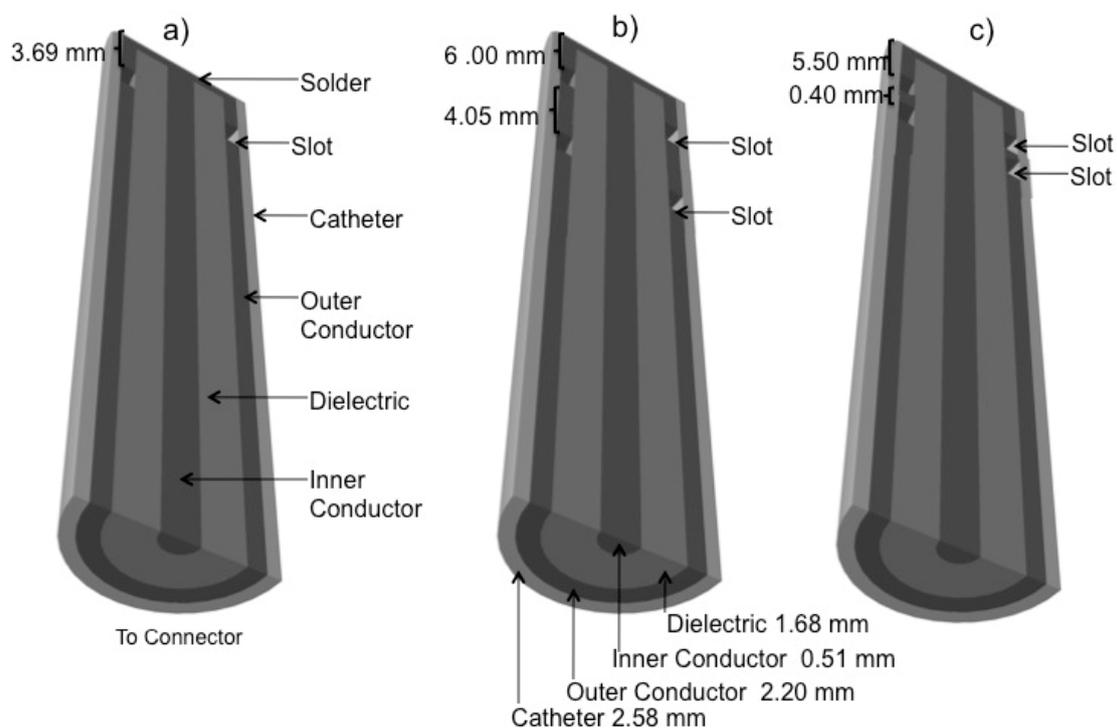
**Figure 1.** Coaxial Slot Antennas. (a) Single slot antenna; (b) Double slot antenna; (c) Double “short-distance” slot antenna.
