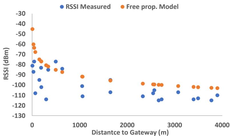
Figure 18. Results of RSSI as a function of the distance.
