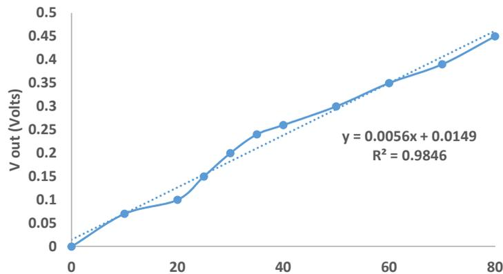
Figure 11. Calibration of anemometer.
