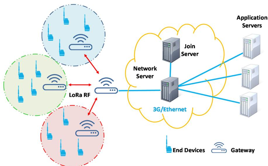
Figure 3. LoRaWAN network architecture.
