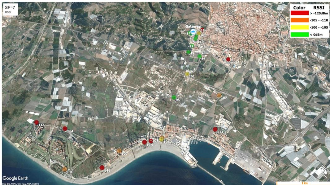
Figure 17. Results of RSSI measured in the scenario.
