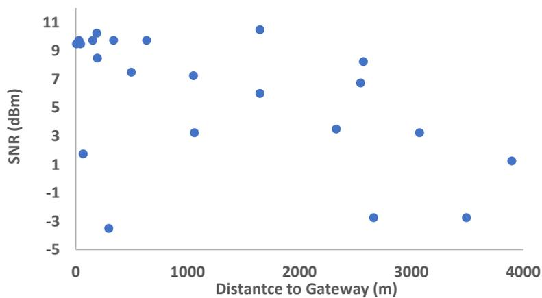
Figure 19. Results of SNR as a function of the distance.
