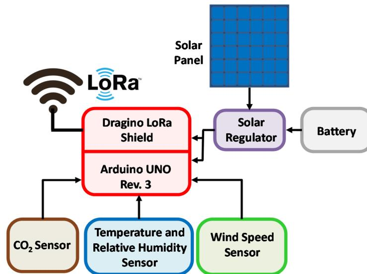
Figure 7. Block Diagram of node components.
