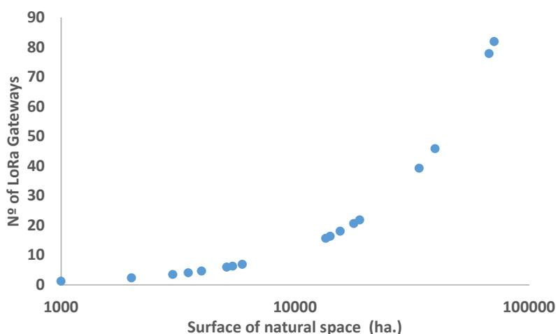
**Figure 26.** Required gateways as a function of the surface.
