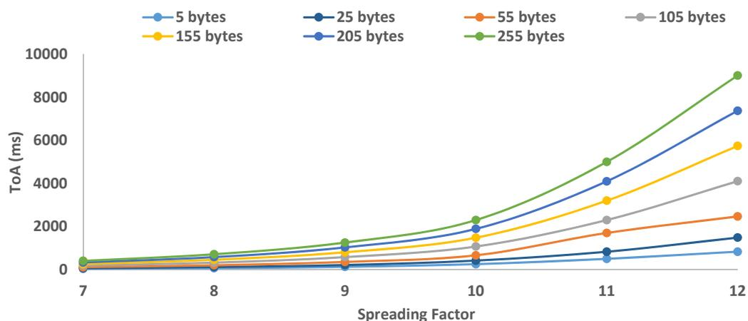
Figure 4. ToA (in ms) for different SF using a bandwidth of 125 kHz.
