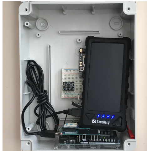
Figure 1. A node of the developed system enclosed in its protective case, along with its battery.
