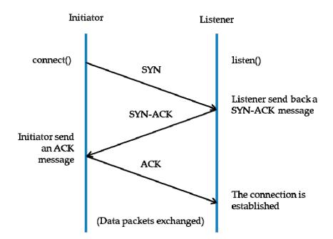
Figure 1. Normal Transmission Control Protocol (TCP) 3-Way Handshake.
