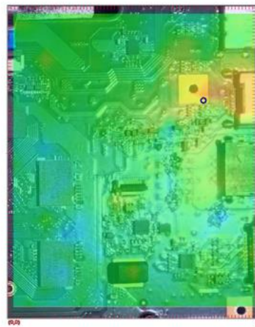
Figure 18. Intensity distribution of the near field after HDMI layout improvement.
