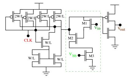
Figure 3. Circuit diagram of the proposed VTC.
