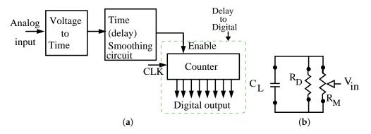
Figure 2. (a) Proposed voltage to time converter (VTC)-based ADC (b) Fundamental Model.
