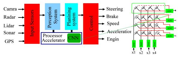
**Figure 1.** Vehicle automation system and use of convolution network-based accelerator using analog to digital converter (ADC).
