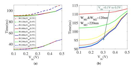
Figure 7. Optimization of (a) the transistor widths of controlling circuit and (b) biasing voltage (V<sub>bb</sub>).
