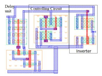
Figure 4. Layout diagram of the proposed VTC.
