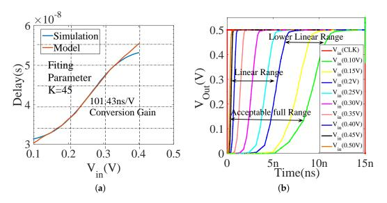
Figure 5. (a) V-T conversion characteristics (b) Output vs. time curve.
