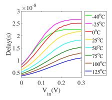
Figure 6. V-T characteristics of VTC for different temperature.
