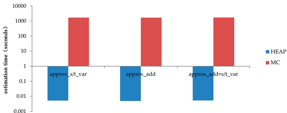
Figure 7. Estimation speed comparison between *HEAP* and MC.
