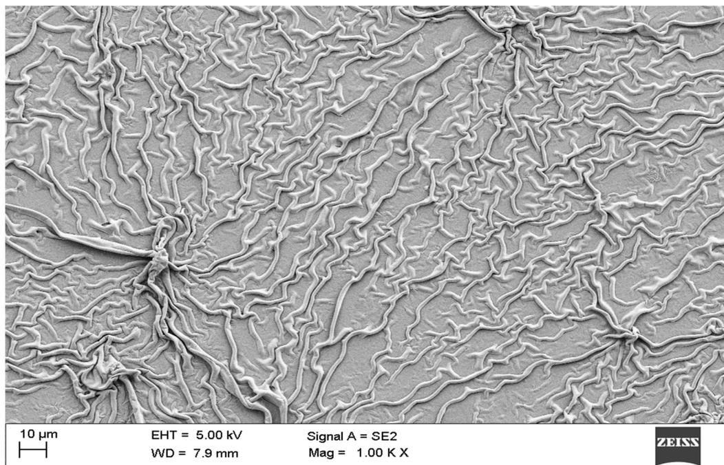
**Figure 2.** SEM image deep UV prepared zinc precursor (ZnO)–rGO thin film. rGO: reduced graphene oxide.
