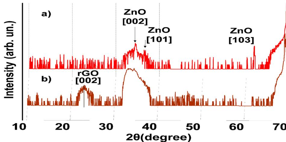
Figure 3. XRD pattern of (a) ZnO thin film and (b) ZnO-rGO thin film.
