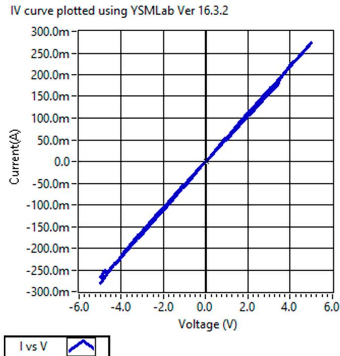
**Figure 5.** Benchmark test result for parasitic effects due to the -V measurement set-up: I–V curve for the FTO sample.
