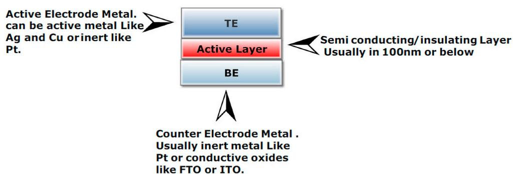
**Figure 1.** Memristor device structure. TE, top electrode; BE, bottom electrode; FTO, fluorine-doped tin oxide; ITO, Indium-doped tin oxide.
