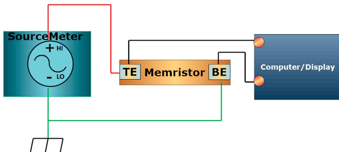
Figure 4. Setup block diagram for current-voltage (I-V) measurements.
