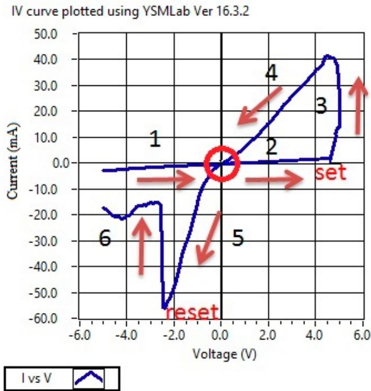
**Figure 6.** Device I–V plot, for a DC sweep cycle in the range  $\pm 5$  V at a sweep rate of 0.5 V/s. The arrow shows the direction of the current.
