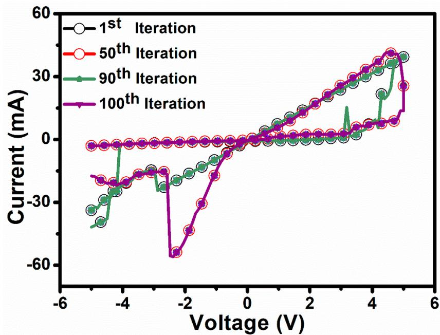
**Figure 7.** Device I–V plot, for a 100 continuous DC sweep cycle in the range of  $\pm 5$  V at a sweep rate of 0.5 V/s.
