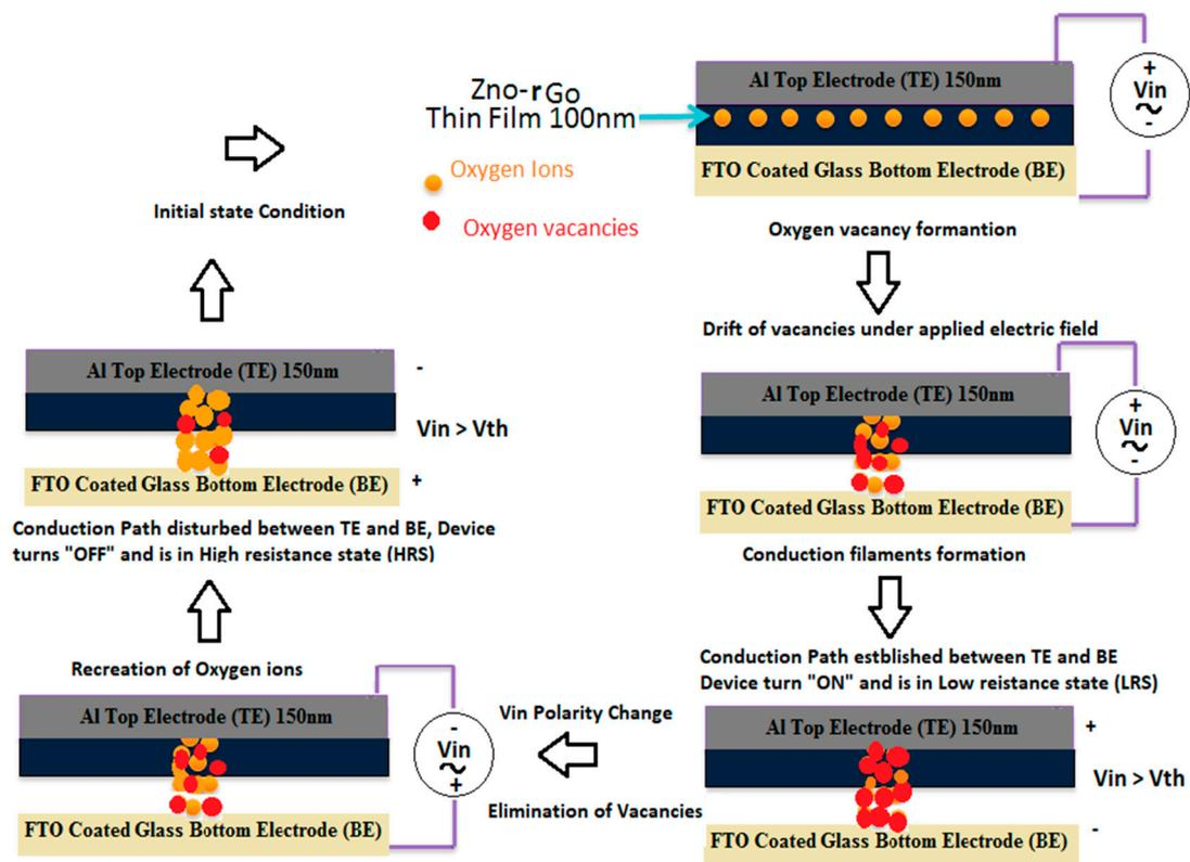
Figure 10. Switching mechanism for the Al-ZnO-rGO-FTO device.
