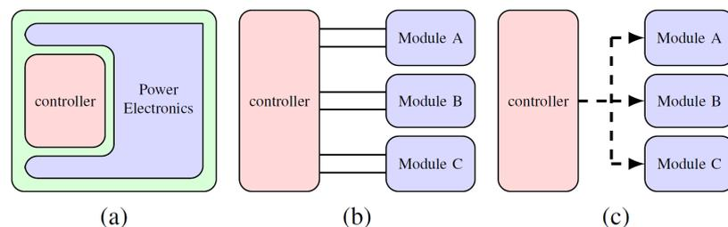
**Figure 1.** Different modular drive configurations: (a) Single Inverter; (b) Direct Gate driving; and (c) Distributed Gate Driving (solid lines represent direct gate connections, dashed arrows represent communication channels).
