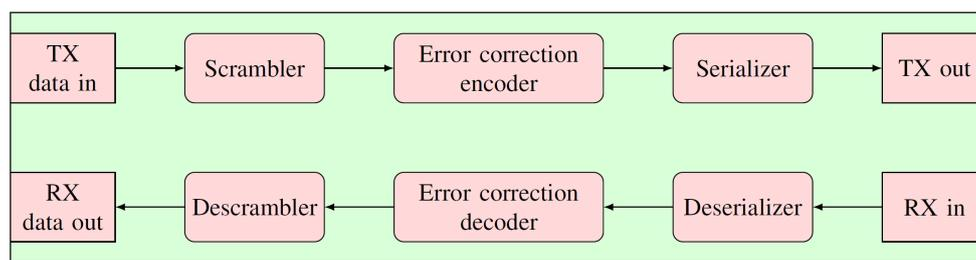
**Figure 2.** Diagram of the overall communication chain.
