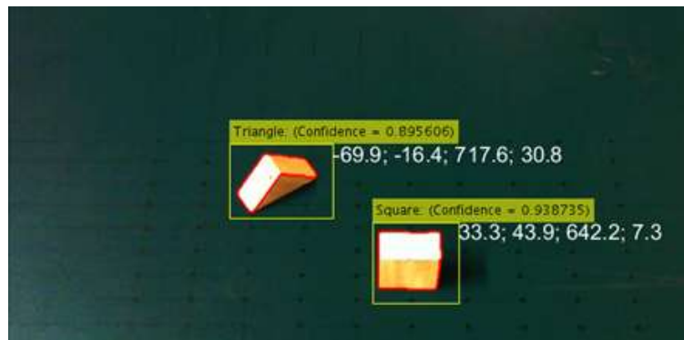
Figure 14. Estimation results of two object names and positions and their orientations.
