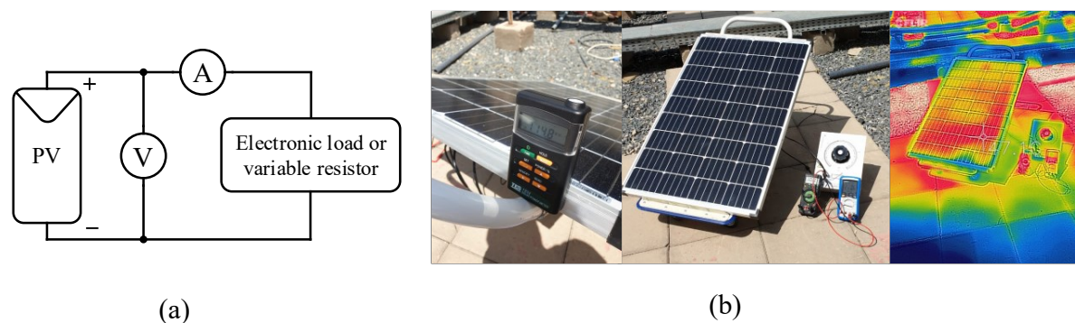
Figure 9. The approach used to produce the dataset for neural network training: (a) schematic diagram of the circuit (b) experimental setup. The electronic load used to sweep the voltage and get the I-V characteristic curve at specific irradiance and temperature values.
