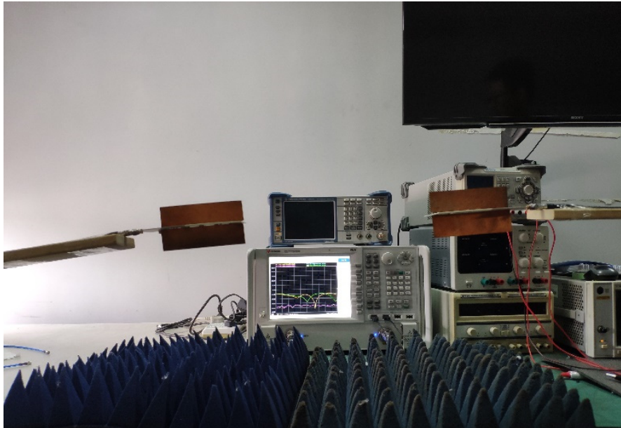
Figure 14. The measurement setup for the phase and magnitude difference.
