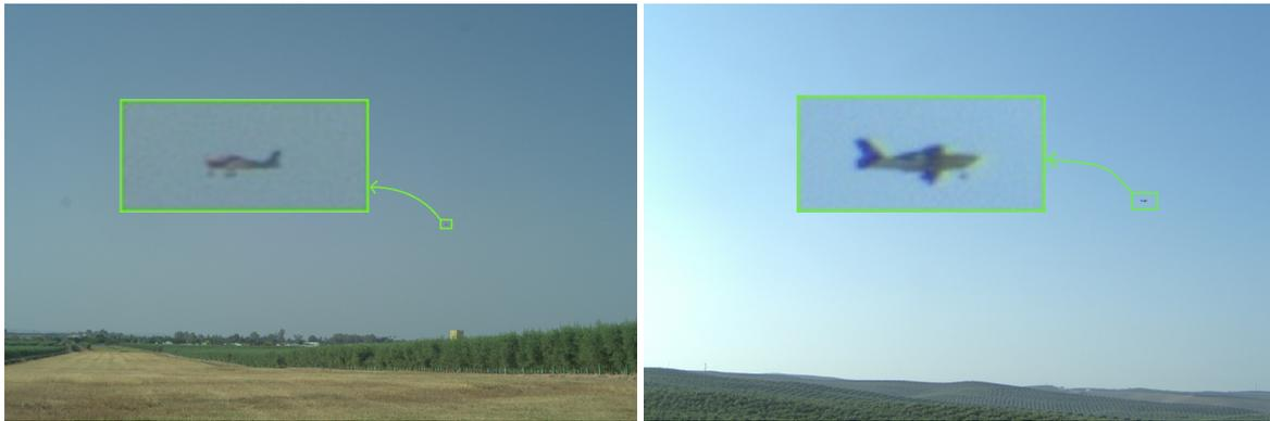
**Figure 1.** Images captured from the ground-based system, showing a small aircraft (SOCATA TB9) flying at a distance of two kilometers. Image resolution:  $5472 \times 3648$  (20 MP); angle of view:  $32.9^\circ$  (horizontal) and  $24.8^\circ$  (vertical). Long-range detection poses a challenge to both image and audio-based strategies.
