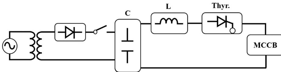
Figure 14. Experimental setup for MCCB interruption phenomena analysis.
