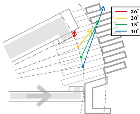
Figure 10. Vector of synthetic force according to the angle between contacts.
