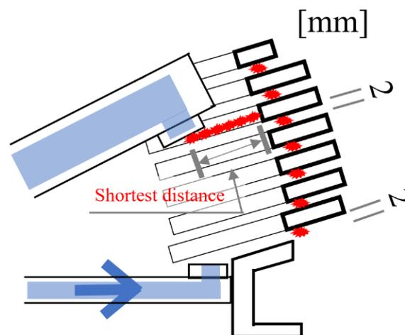
Figure 11. The shortest distance between the arc and splitter plate in basic state.
