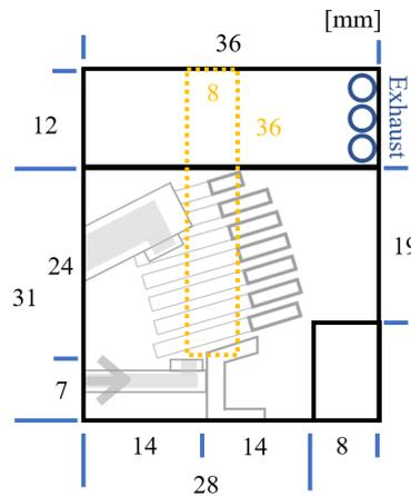
Figure 8. MCCB interior space and virtual space for hot gas movement (side view).
