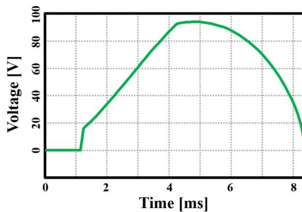
Figure 6. Voltage waveform between contacts without a splitter plate.
