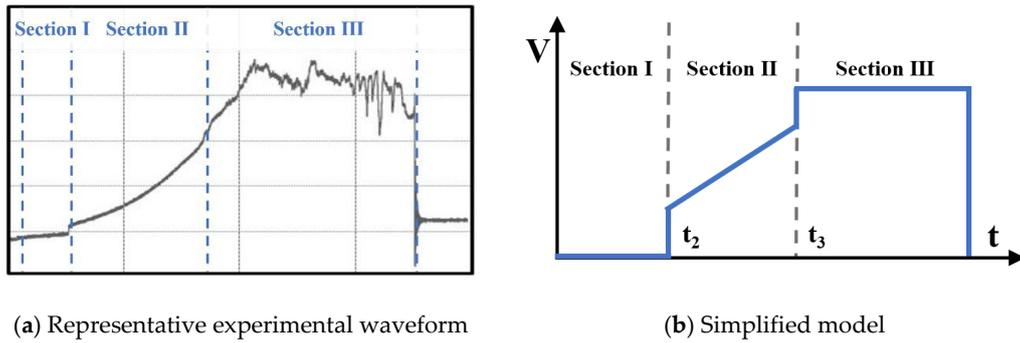
Figure 1. Molded case circuit breaker (MCCB) interruption voltage.
