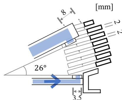
Figure 5. Structure and dimensions of the contacts and splitter plate.
