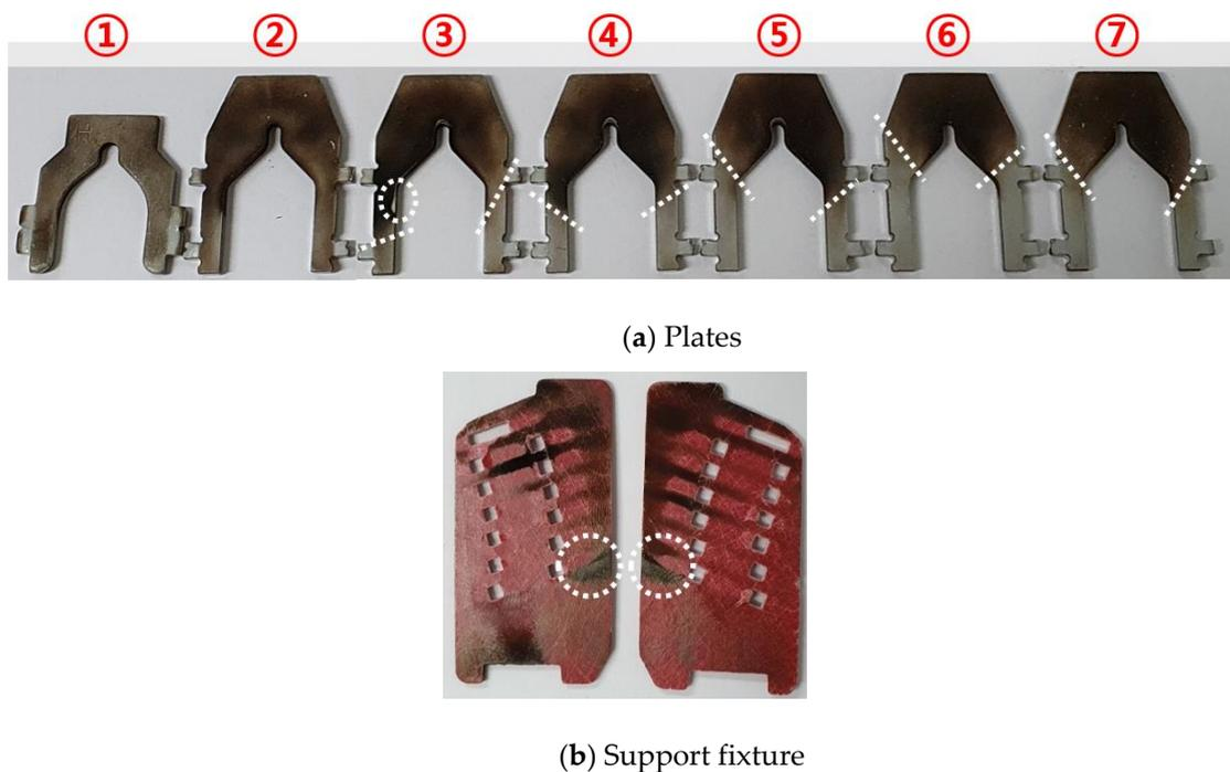
**Figure 16.** Damaged splitter plate after experimentations.
