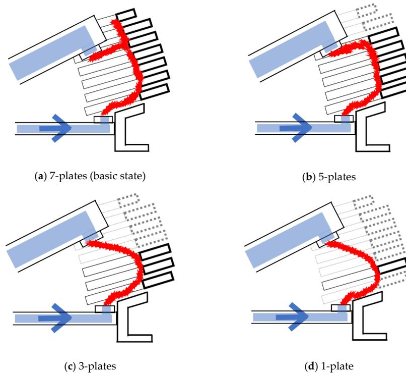
Figure 4. Splitter plate change cases for MCCB modeling.
