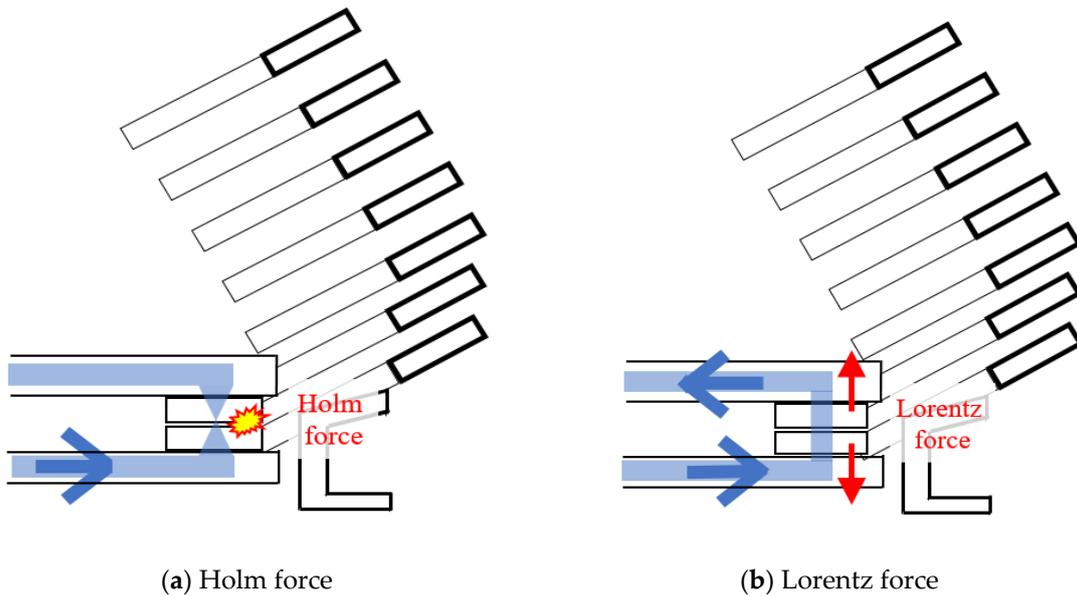
Figure 2. Electrodynamic repulsion force generated in the MCCB.
