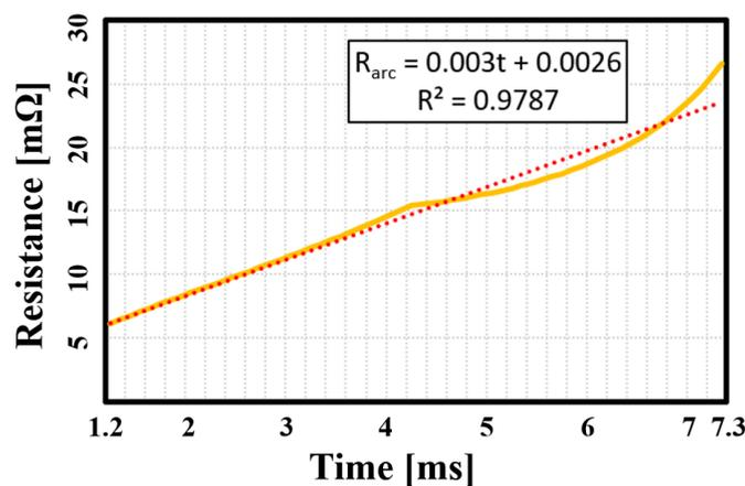
Figure 7. Resistance ( $R_{arc}$ ) between the contacts in section II.
