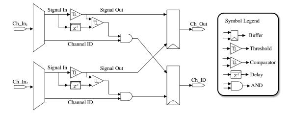
Figure 4. System architecture for a channel activation register unit with 2 input channels.
