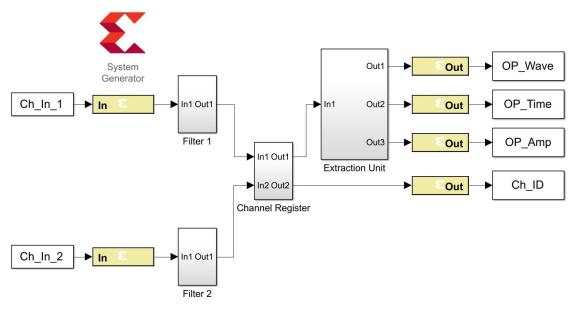
Figure 8. Design of a multichannel unfiltered input system (MCUF) in SysGen.
