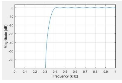
Figure 2. Frequency response of the neural signal FIR filter.
