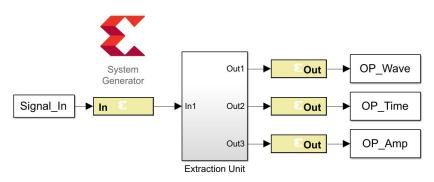
Figure 5. Design of a single-channel filtered input system (SCF) in SysGen.
