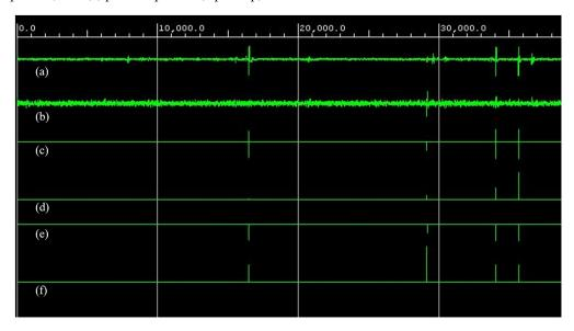
**Figure 11.** Waveforms from the multichannel (two-channel) filtered input system: (**a**) input signal from Channel-1 (Ch\_In\_1), (**b**) input signal from Channel-2 (Ch\_In\_2), (**c**) output wave during neural activity (Op\_Wave), (**d**) timestamp (Op\_Time), (**e**) peak amplitude (Op\_Amp) and (f) channel identification (Ch\_ID).
