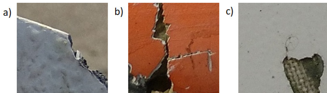
Figure 2. Example of rotor blades with defects: (a) fracture; (b) crack; and (c) chipping.
