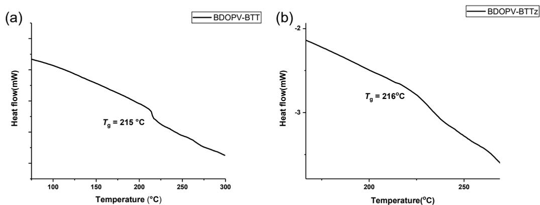
**Figure S2.** Differential scanning calorimetry (DSC) curves of the copolymers. All the DSC curves are the second heating and cooling processes under nitrogen flow ( $50\text{ mL min}^{-1}$ ) at the scan rate of  $10\text{ }^{\circ}\text{C min}^{-1}$ .
