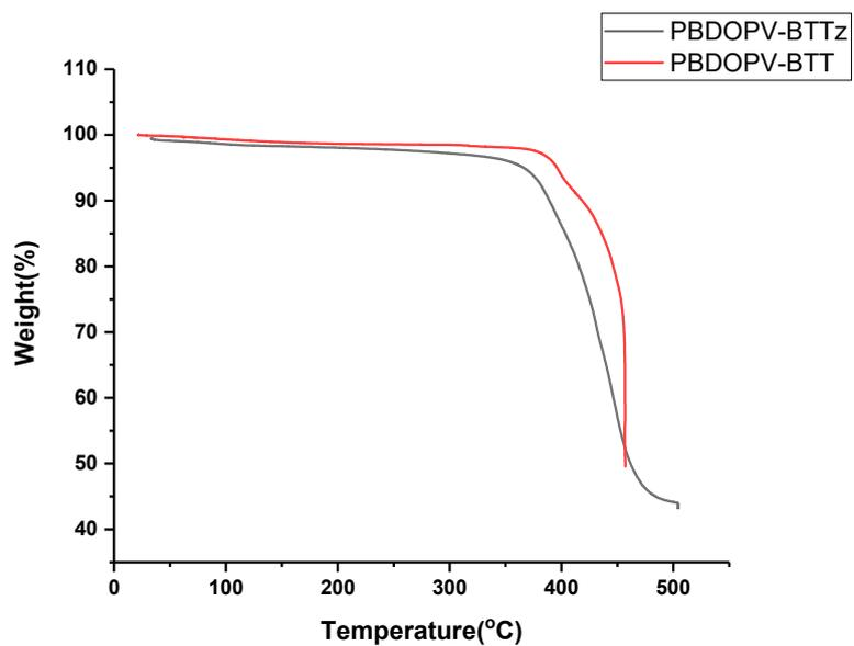
**Figure S1.** Thermogravimetric analysis (TGA) curves of the copolymers under nitrogen atmosphere at the heating rate of  $10\text{ }^{\circ}\text{C min}^{-1}$ .
