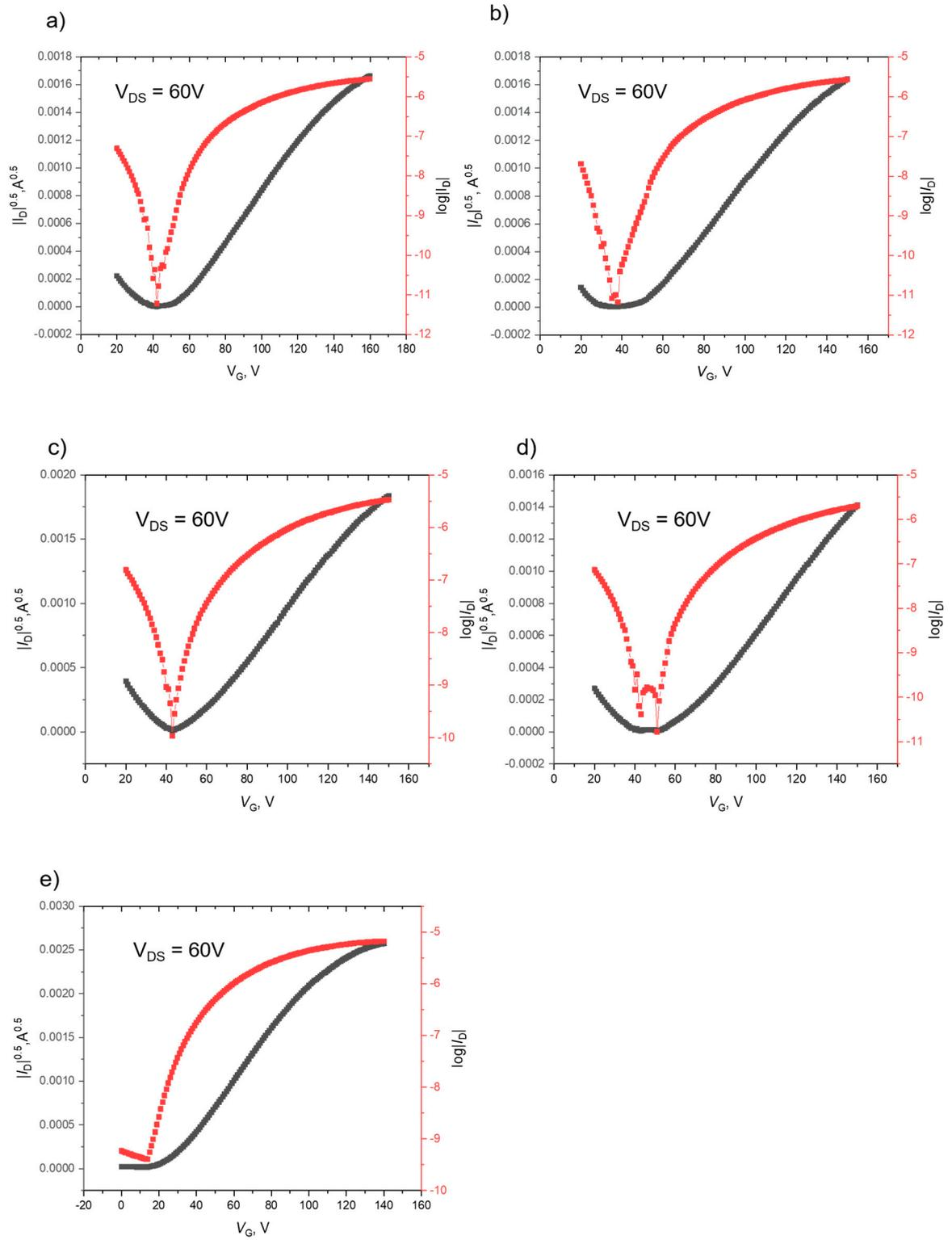
**Figure 3-1.** Transfer curves of thin film transistors based on PBDOPV-BTT: (a) as cast, after thermal annealing at (b) 150 °C, (c) 180 °C, (d) 210 °C, and (e) 240 °C ( $L = 100$  m and  $W = 1000$  m).
