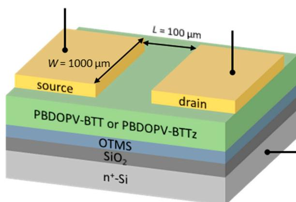
**Figure S4.** Schematic illustration of the thin film transistor structure, where  $n^+$ -Si is a heavily  $n$ -doped Si wafer coated with a  $\text{SiO}_2$  layer, OTMS is octadecyltrimethoxysilane self-assembly monolayer, source and drain electrodes are vacuum-deposited Au,  $W$  and  $L$  are channel width and length, respectively.
