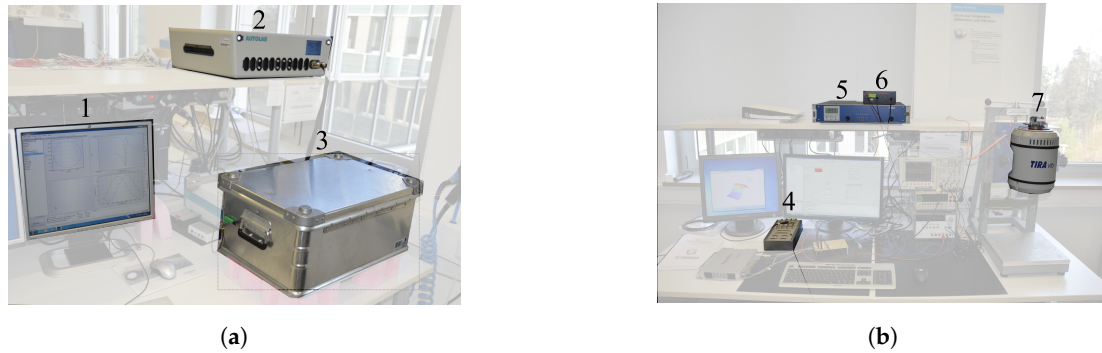
Figure 2. (a) Equipment used for the characterization of the PEG and first tuning at Fraunhofer IIS; (1) NOVA 1.10 software, (2) potentiostat/galvanostat -Autolab PGSTAT302N, and (3) Faraday cage. (b) Equipment used for performing the second tuning and the testing with the real vibration signal: (4) dSPACE DS1104, (5) power amplifier TIRA BAA120, (6) programmable resistance decade box developed at Fraunhofer IIS, and (7) Electrodynamic shaker TIRA S52110.
