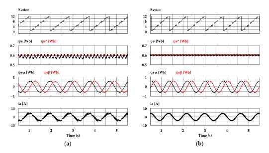
**Figure 7.** Sectors, stator flux,  $\alpha$ - $\beta$  components of stator flux and stator current responses of five-level HTR at 50 r/min in the forward direction of IM: (a) Classical DTC; (b) proposed DTC-SFRS.
