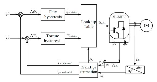
Figure 3. Complete structure of a classical DTC.
