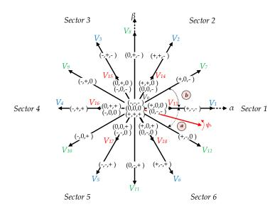
**Figure 2.** Space vector representation of three-level NPC inverter.
