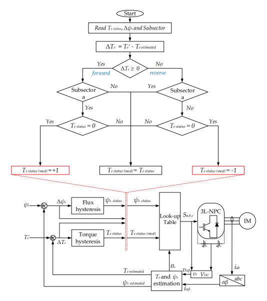
Figure 6. The complete structure of the proposed DTC-simple flux regulation strategy (SFRS).
