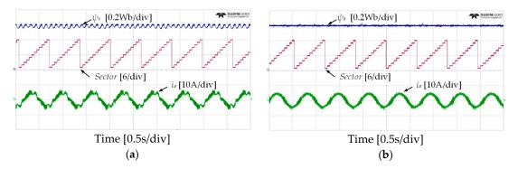
**Figure 10.** Stator flux, sectors and current responses of five-level HTR at 50 r/min in forward direction of IM: (a) classical DTC; (b) proposed DTC-SFRS.
