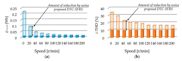
**Figure 18.** Effectiveness of the proposed method at different speed operations: (a) Minimizing stator flux-droop; (b) reducing stator current THD.
