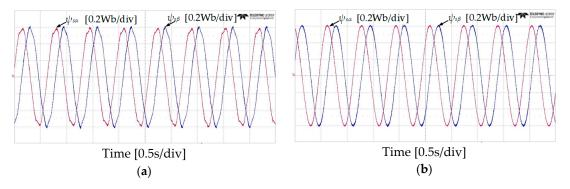
**Figure 12.**  $\alpha$ -β components of stator flux responses of five-level HTR at 50 r/min in forward direction of IM: (a) classical DTC; (b) proposed DTC-SFRS.
