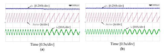
**Figure 16.** Speed transient from 150 r/min to 50 r/min: stator flux, sectors and current responses of five-level HTR in forward direction of IM: (a) classical DTC; (b) proposed DTC-SFRS.
