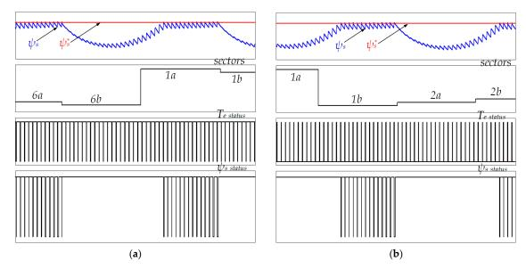
**Figure 5.** Sector flux-droop of the induction motor (IM) at low-speed: (a) Forward direction; (b) reverse direction.
