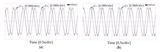
**Figure 13.**  $\alpha$ - $\beta$  components of stator flux responses of five-level HTR at 50 r/min in reverse direction of IM: (a) classical DTC; (b) proposed DTC-SFRS.
