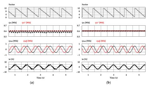
**Figure 8.** Sectors, stator flux,  $\alpha$ - $\beta$  components of stator flux and stator current responses of five-level HTR at 50 r/min in reverse direction of IM: (a) Classical DTC; (b) proposed DTC-SFRS.
