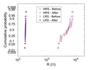
**Figure 8.** Cumulative distributions of the resistance values for a single RRAM ( $2 \times 2 \mu m^2$ ) before and after a single laser pulse. The spot size is 3  $\mu m$ .
