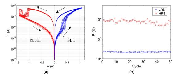
**Figure 3.** (a) DC resistive switching behavior during successive SET and RESET operations; and (b) High resistance state (HRS) and low resistance state (LRS) extracted from the DC resistive switching behavior.at -0.1 V and +0.1 V, respectively.
