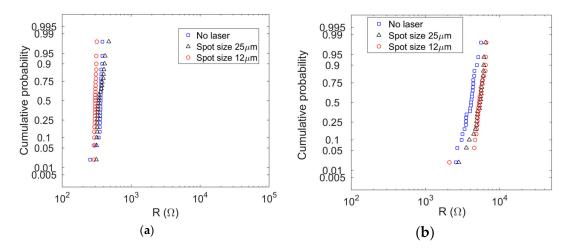
**Figure 7.** Cumulative distributions of the resistance values for a single RRAM ( $5 \times 5 \mu m^2$ ) before and after a single laser pulse for different spot sizes (**a**) RRAM in the LRS; and (**b**) RRAM in the HRS.
