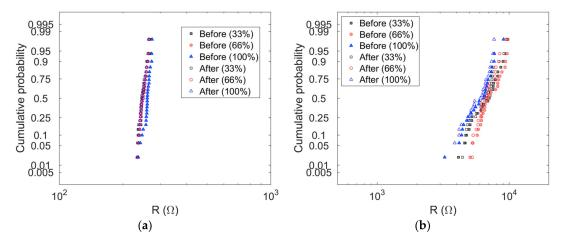
**Figure 5.** Cumulative distributions of the resistance values for a RRAM ( $15 \times 15 \mu m^2$ ) before and after a single laser pulse (spot size of  $25 \mu m$ )., sweeping the power source value (**a**) RRAM in the LRS (**b**) RRAM in the HRS.
