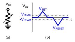
Figure 2. (a) Schematic device measurement configuration; and (b) Diagram of the applied voltage ramps.
