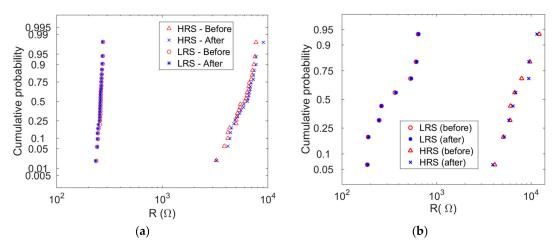
**Figure 6.** Cumulative distributions (a) of the resistance values for a single RRAM (15  $\times$  15  $\mu$ m<sup>2</sup>) before and after a single laser pulse; and (b) of the average resistance for 8 RRAMs of different sizes (152 devices of 2  $\times$  2  $\mu$ m<sup>2</sup>, 3 of 5  $\times$  5  $\mu$ m<sup>2</sup> and 3 of 15  $\times$  15  $\mu$ m<sup>2</sup>) before and after a single laser pulse. The spot size is 25  $\mu$ m.
