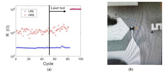
**Figure 9.** (a) Equivalent resistance for a RRAM during the experiment where the laser source released energy continuously; and (b) Photograph of the RRAM after the experiment.
