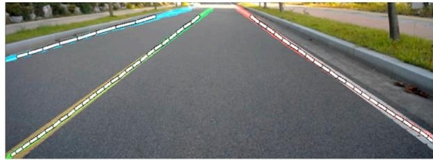
Figure 7. Lane detection by SSCNN.
