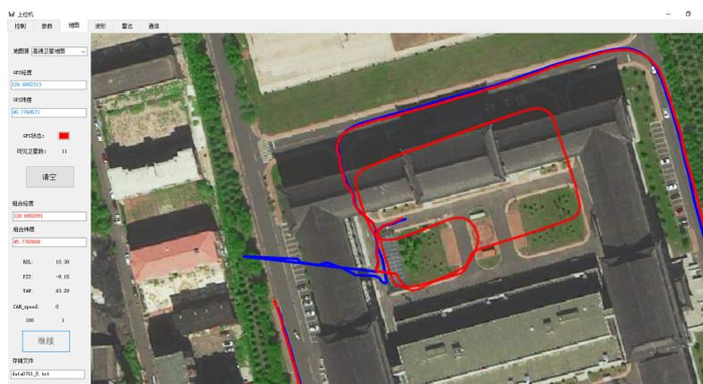
Figure 10. GPS-MEMS EKF trajectory comparison diagram.
