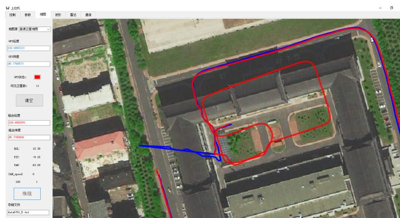
**Figure 10.** GPS-MEMS EKF trajectory comparison diagram.
