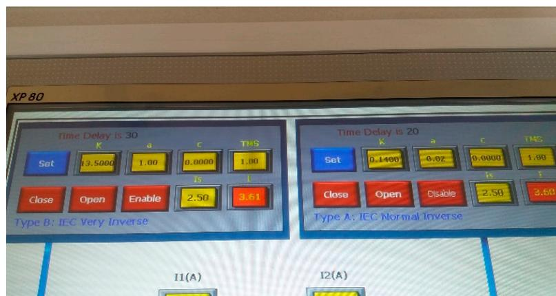
Figure 17. Two relays mode of operation (relay upgrading).
