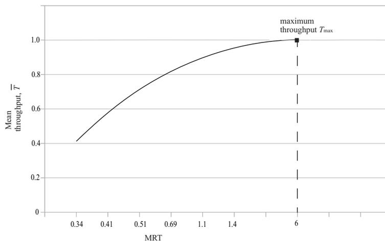
**Figure 3.** Relationship between MRT and mean throughput.
