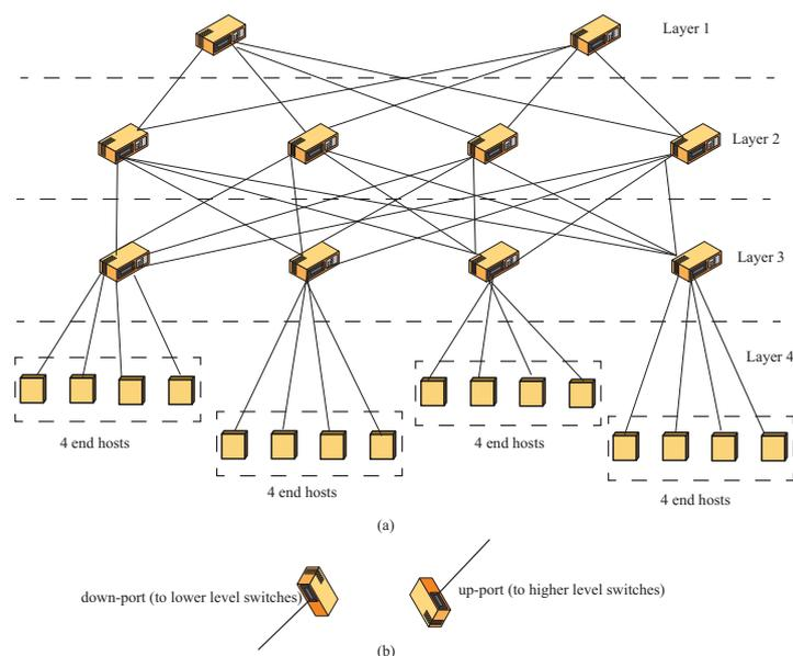
**Figure 1.** (a) A three layer fully-populated network, (b) Up and down ports.
