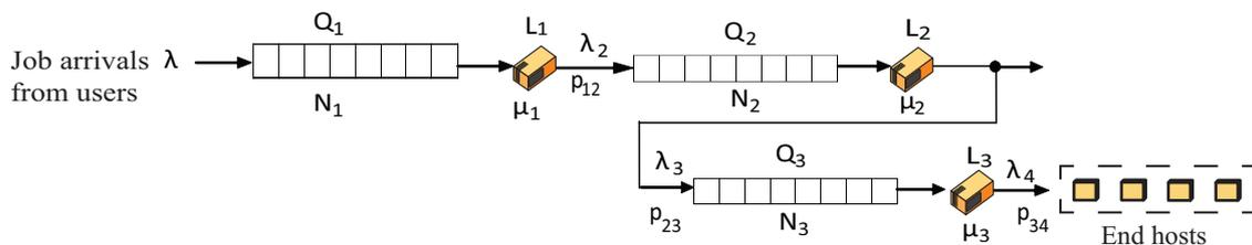
**Figure 2.** The interconnections of the Fully-Populated Network (FPN) of Figure 1, as depicted from the Probabilistic Model (ProMo) point of view.
